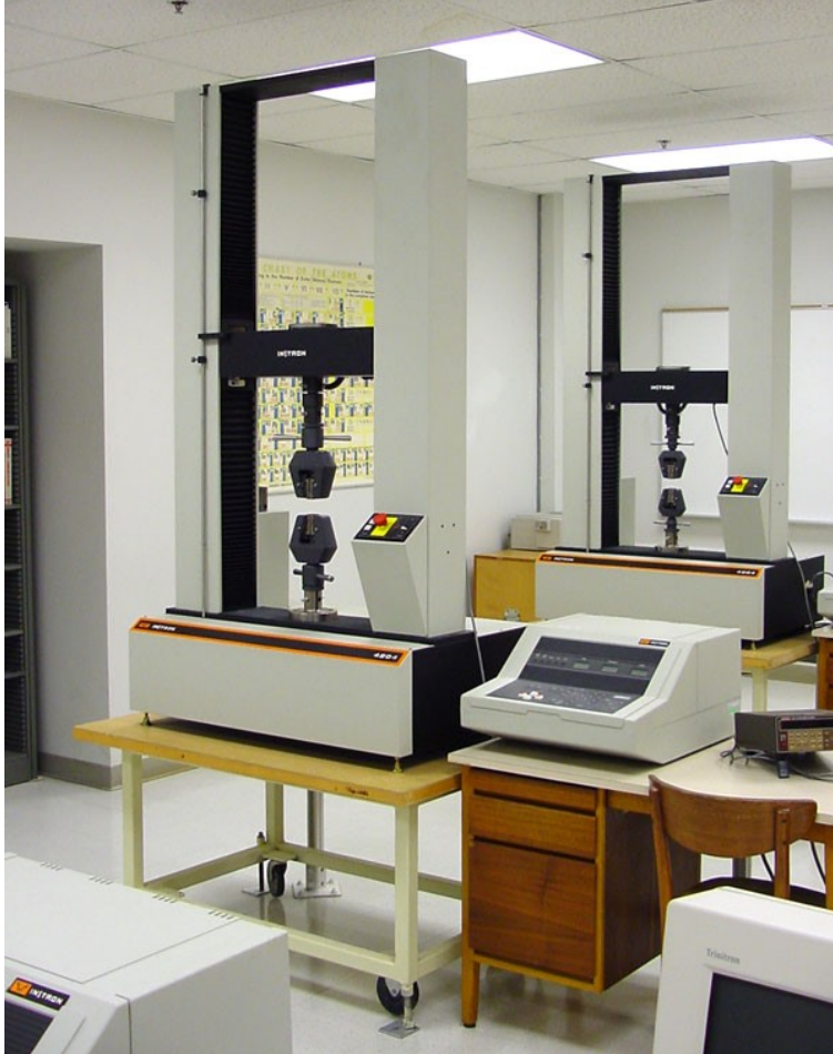
Instron 4204 Universal testing system
