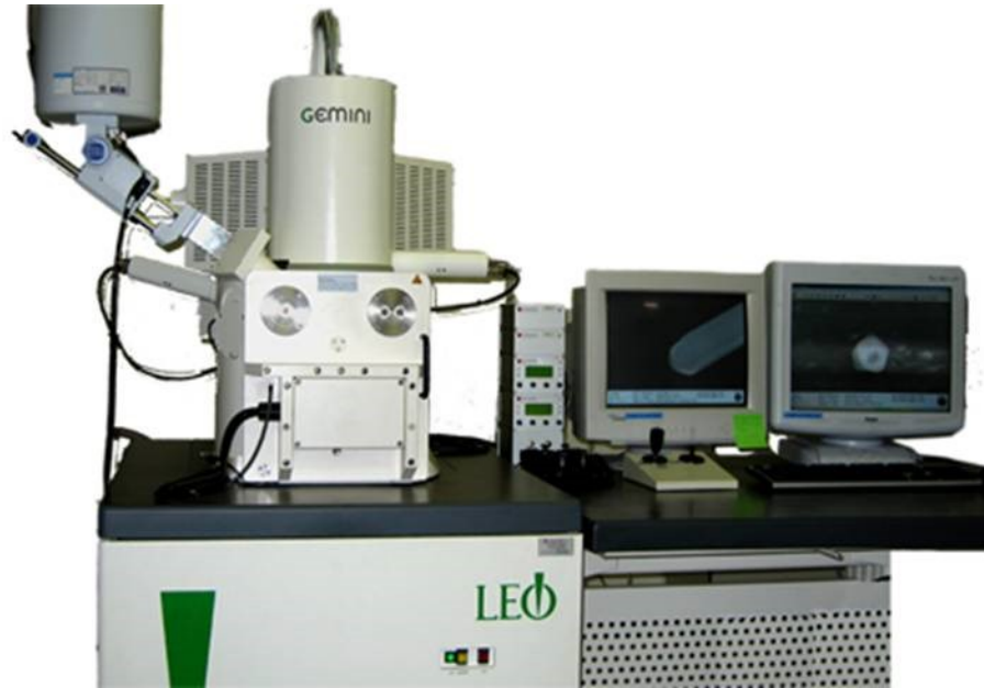
LEO 1525 FE-SEM with EDX probe Bruker Field Emission Scanning Electron Microscope
