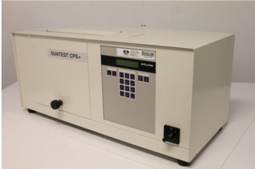
Suntest CPS+ Atlas Xenon Test Instrument
