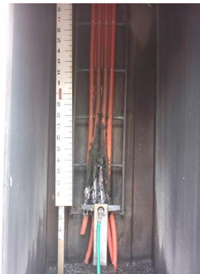
Composite materials show a considerable increase in the degradation temperature and a **flame retardant** effect due to the presence of a char layer formed during the combustion. This char layer is an inert and insulating coating which acts as a physical barrier between the polymer and the combustion environment.
